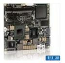
ETX® - Highly integrated, PC-compatible embedded modules based on x86 CPU architecture – all that on a footprint of 95 x 114 mm.
